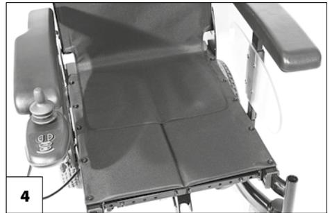
The extended parts of the back support are fastened to the top or bottom seat surface depending on the adjusted back support height (4).
